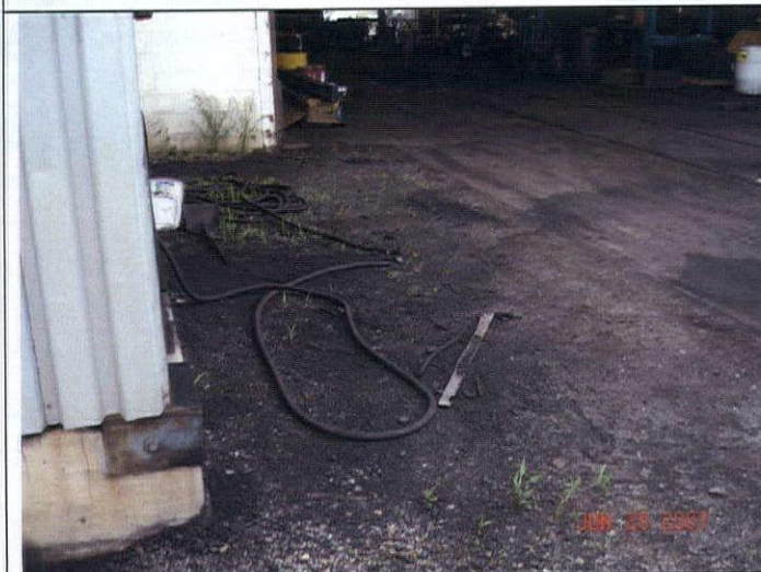
Hose left outside of the containment structure for the used anti-freeze and oil near the northern maintenance area. All hoses should be stored inside of the containment to prevent leaks and spills.
