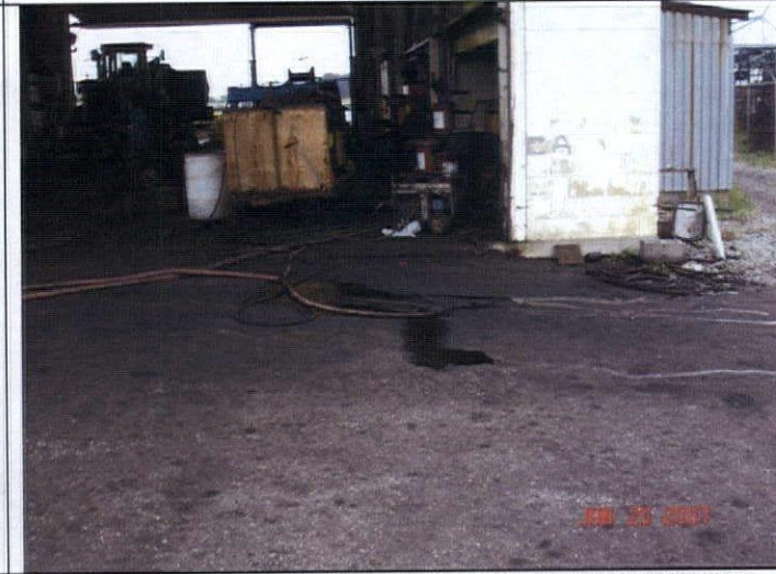
Shop area with water runoff. There is also a steam cleaner in the shop area. All discharges from this area should be contained and not sent to the ponds.
