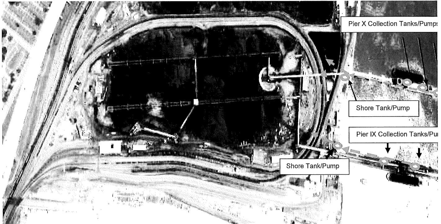
NOTE: Pier X storm water collection system is currently inoperable. The under pier piping system has sustained severe damage from debris in the river at high tide.
