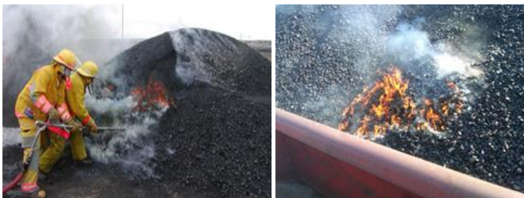
Figure A1.2. Glowing combustion in coal stockpile (left). Flaming combustion of coal in a cargo ship (right)
